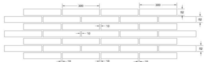
ELEVATION SHOWING THE FIRST KIND OF BRICK COURSES
